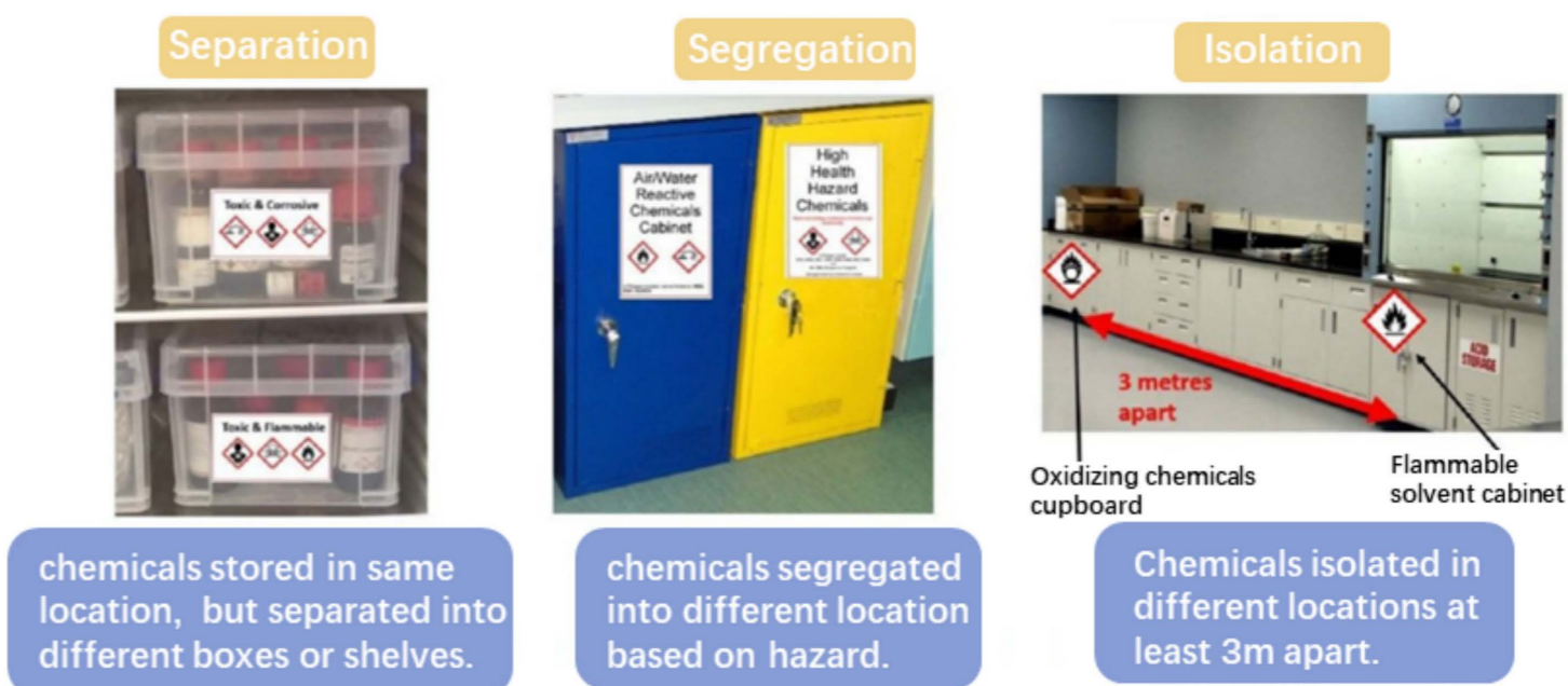
Figure 2. Principles of chemical separation (a), segregation (b), and isolation (c) [2] .
